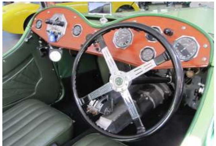
Cockpit detail. The LH knob is the idle setting, RH is the on-off-reserve fuel tap and upper RH is the choke. Note the stubby preselector gearshift. Handbrake is off course fly off and the intrusion at the top left is the temporarily mounted air/fuel meter.
