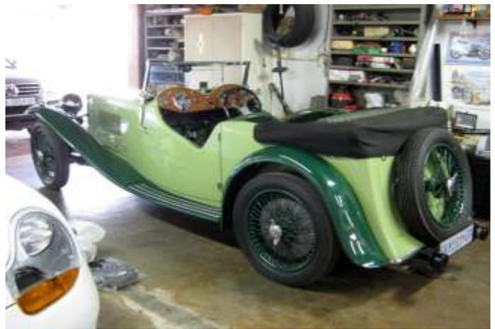
Remove the spare, fold out the boot tray on its arms, reinstall the spare and strap luggage to the boot tray. Note the size of the brake drums.
